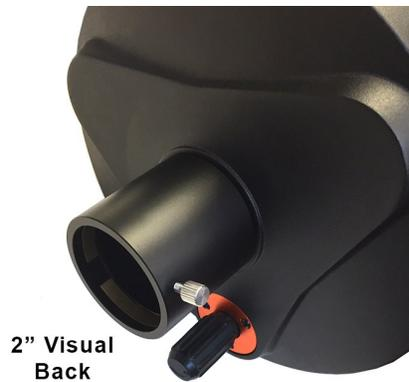
The Night Owl simply slides into the 2" visual back and is held by a thumbscrew and clamping ring. The position of the reducer lens relative to the telescope is not critical, but sliding the lens in as far as possible will give the nominal .4x reduction factor.
