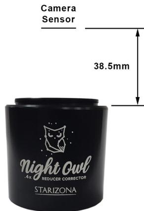
The Night Owl has standard T-threads on the camera side, so you simply need to add the correct length T-thread spacers to adapt most cameras. For example, when using a ZWO cooled camera, which has a backfocus of 17.5mm, you need a 21mm spacer, which is one of the adapters included with the ZWO camera.
