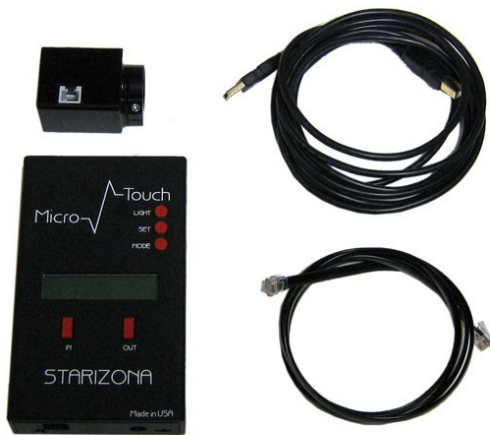
Hand control, motor, cables
