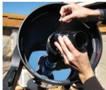
Mounting the HyperStar lens system to a Schmidt-Cassegrain telescope takes minutes.
