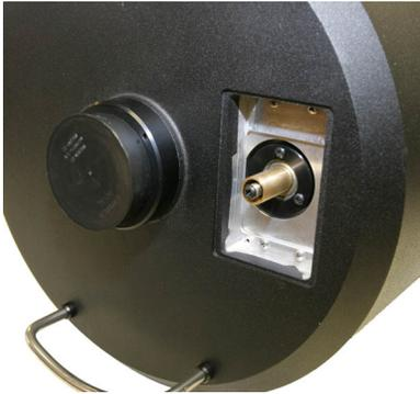
Turn the brass focus shaft clockwise to bring the mirror back and expose the Phillips-head screw at the end of the threaded focus rod.
