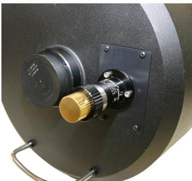
Use the three included hex-head screws to attach the SCT MicroFocuser to the telescope. You are now ready to head out under the stars!
