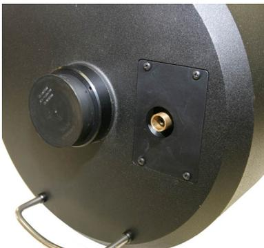
Begin by pulling off the rubber focus knob exposing the brass shaft underneath, as shown above.
