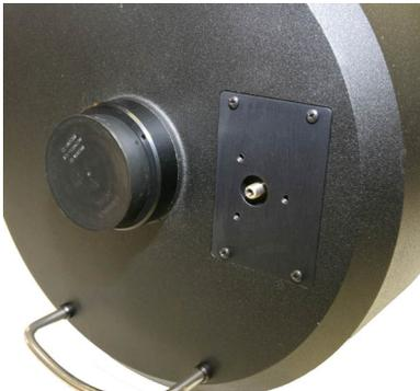
Use the original 4 screws to attach the included adapter plate. Be sure the beveled side is in toward the telescope. There is only one proper orientation for the plate, with the large hole on the left side.
