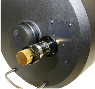
Begin threading the SCT MicroFocuser onto the threaded focus rod. When there is only about 1/4" left to go, simply push the focuser the rest of the way in. This will take up some of the focus travel from when you removed the original focuser, making it quicker to return to the proper focus the first time you use your telescope after the SCT MicroFocuser installation.
