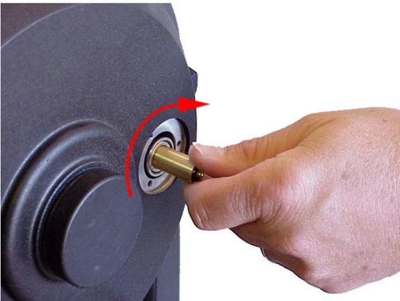
Rotate the brass portion of the focus assembly *clockwise*. This will bring the mirror back and expose the threaded portion of the focus shaft. At the tip of this threaded bolt will be either a small C-clip or a screw which will be removed in the next step.
