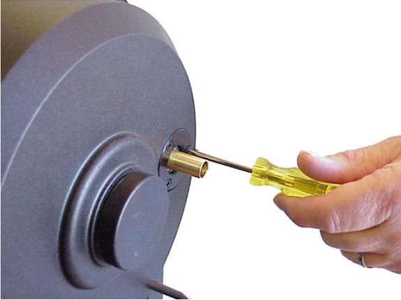
There are 3 small screws which hold the focus assembly cover in place. These will be Phillips-head screws on newer scopes, but some models will have hex-head screws. Remove these screws and take off the flat cover plate, exposing the inside of the focus assembly.
