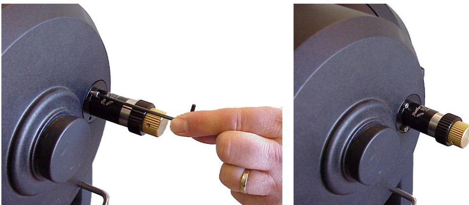
Use the three provided hex-head screws and wrench to attach the SCT MicroFocuser to the telescope. You are now ready to head out under the stars! Use the black knob for coarse focus and the brass knob for fine focus (10:1 ratio).
