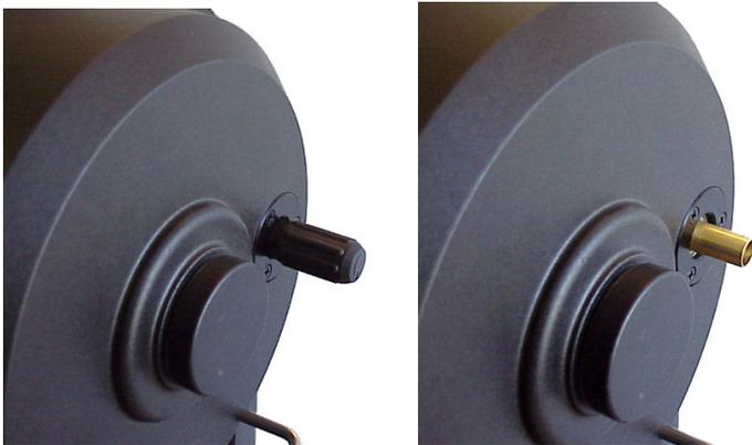
The newest Celestron telescopes have a rubber knob which can be pulled off. Older 8" telescopes will have a metal focus knob which must be removed using a 1/16" hex-head wrench to loosen a small set screw. Once the knob is removed you will see the brass focus shaft as shown in the second picture above.
