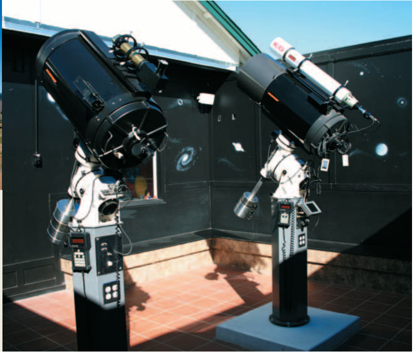
Above: Kiwanis Chico Community Observatory, seen with the future site of the Shoemaker Open Sky Planetarium in the foreground, features a roll-off-roof design. Right: The observatory houses twin Celestron 14-inch Schmidt-Cassegrain telescopes on Astro-Physics computerized mounts. The setup on the right is configured to broadcast digital video images to small displays held by visitors to the outdoor planetarium nearby.
