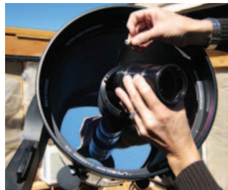
Mounting the HyperStar lens system to a Schmidt-Cassegrain telescope takes minutes.
