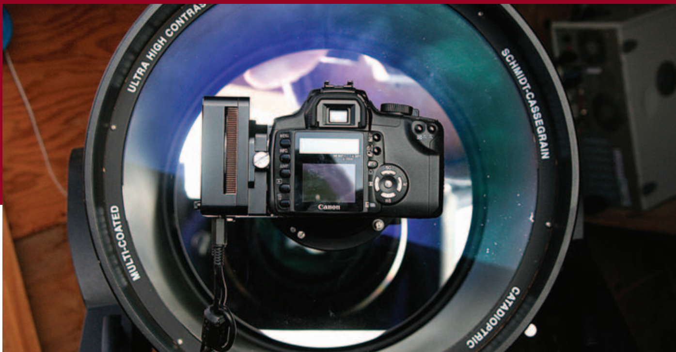
With a Canon digital SLR camera mounted to a HyperStar-ready telescope, the author is equipped for one-shot color astrophotography.
