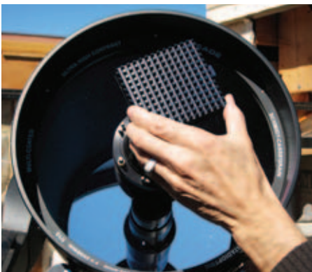
Meade's Deep Sky Imager PRO III camera mounts easily on the HyperStar. This is just one of the many CCD and digital cameras the HyperStar lens system will accept.
